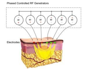
Figure 1. Configuration of six phase controlled RF sources as implemented in the Endymed Pro multisource technology. Multisource RF technology is based on the fact that flow of energy on the surface is minimal, while all energy is directed to the depth of the tissue. This is achieved by repulsion between electrical field of the same polarity on each side of the handpiece.
